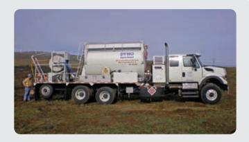
as it is pumped into the borehole. The gassing reaction sensitises the emulsion and expands it to the desired density (from 0.9 to 1.25 grams per cubic centimetre) to optimise blasting results.
