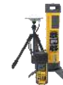
(DGPS) Tagging & Hole Identification using Differential Global Position System
